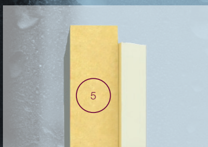
5. High performance core - 0.021 W/mk Thermal Conductivity.
