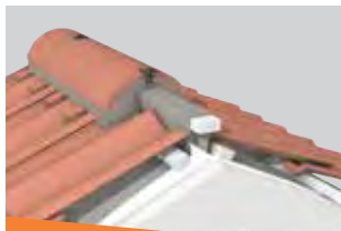
Mortar bedded security ridge
